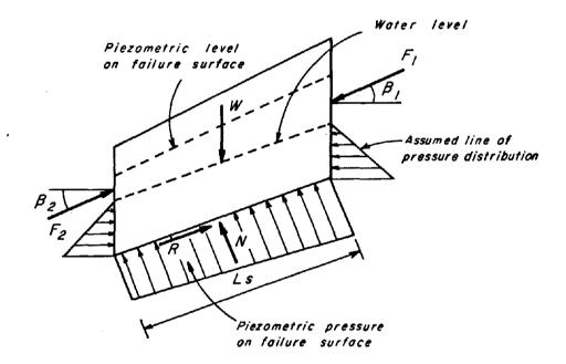
W = total weight of soil and water above the failure surface N = effective reaction normal to the failure surface R = shearing resistance of the soil  $F_1, F_2$  = interelement forces between adjacent slices  $\beta_1, \beta_2$  = inclination of the interelement forces from the normals to the slice faces.
