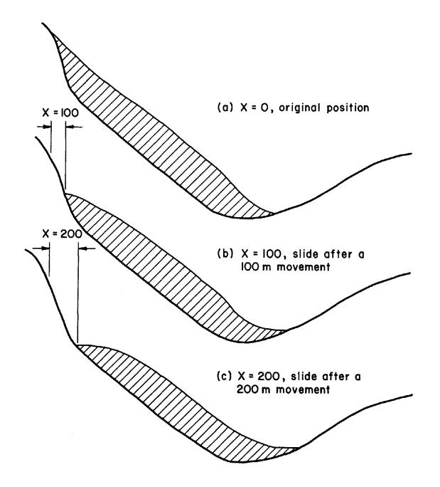
Figure El. Slide at Various Stages of Movement
