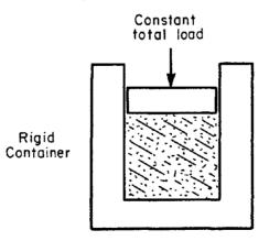
Figure F1. Idealization of vertical deformation with lateral restraint (uniaxial compression test)
