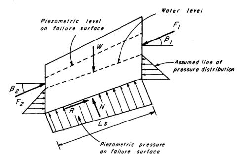
W = total weight of soil and water above the failure surface N = effective reaction normal to the failure surface R = shearing resistance of the soil  $f_1, F_2$  = interelement forces between adjacent slices  $B_1, B_2$  = inclination of the interelement forces from the normals to the slice faces.
